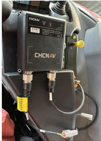
5. Connect to power with NX510 main cable in the tractor cab or tractor battery depending on users.
