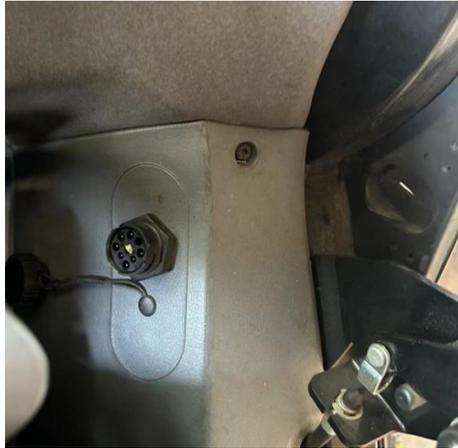
2. Try to find the correct CAN L and CAN H pinouts ( H/J, or C/D)in this interface with tractor documentation or some can tool.
