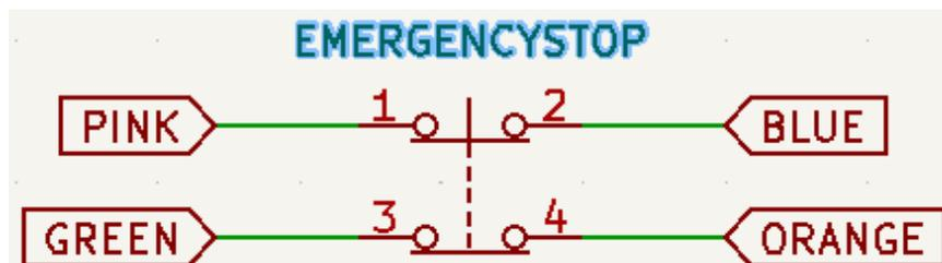
Picture 7: Emergency stop connection diagram
