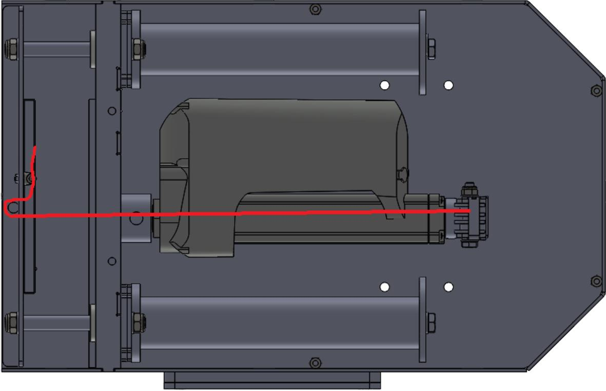
Picture 4: Wire rope route brake module
