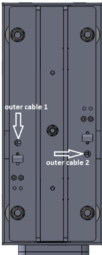
Figure 5: mounting points outer cable brake module
