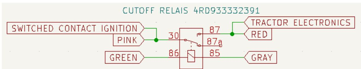
Picture 11: Relay tripping connection diagram
