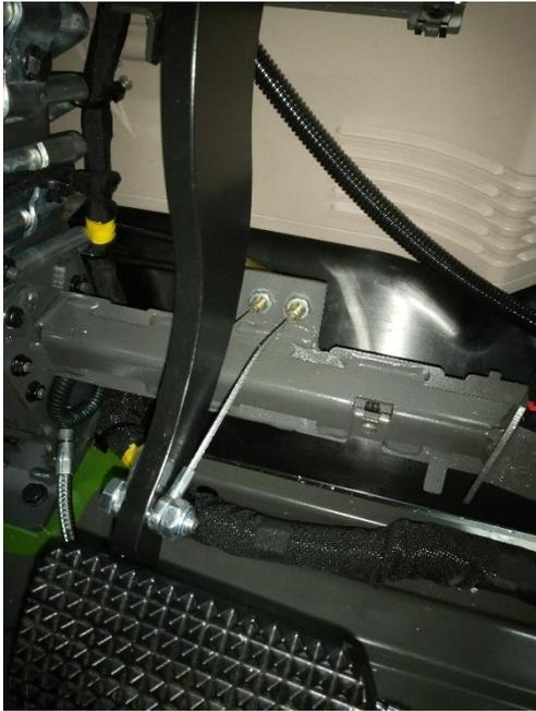
Make sure that the brake cables do not make sharp turns, as this will cause the cables to be damaged or to run too stiffly. The 2 round eyelets must be mounted on the pedals. Use a through-bolt to secure the eyelet rounds to the pedals. See the image on the left for an example. The inner cable must run as straight as possible to the outer cable, otherwise this cable will be damaged too much.
