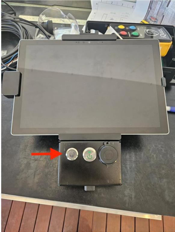
Picture 10: Roadswitch mounted in the switch bracket.
