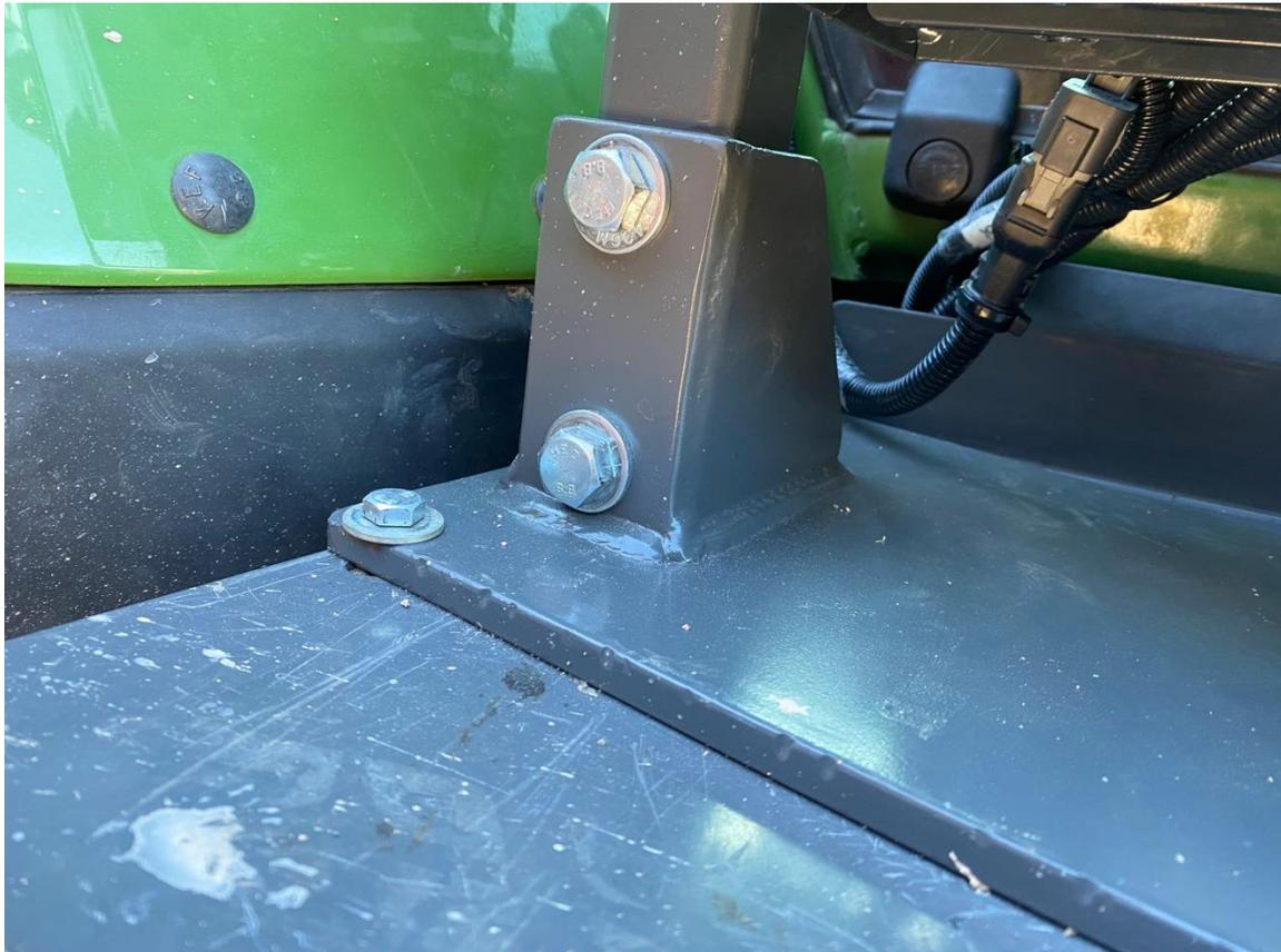
*Picture 2: VDM Base Plate and VDM mounted in sockets.*
