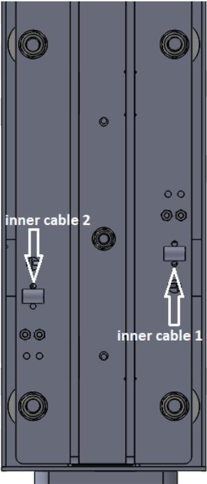
Assemble the cables through the bottom of the brake module and secure the cable with the 2 radius wire clamps.
