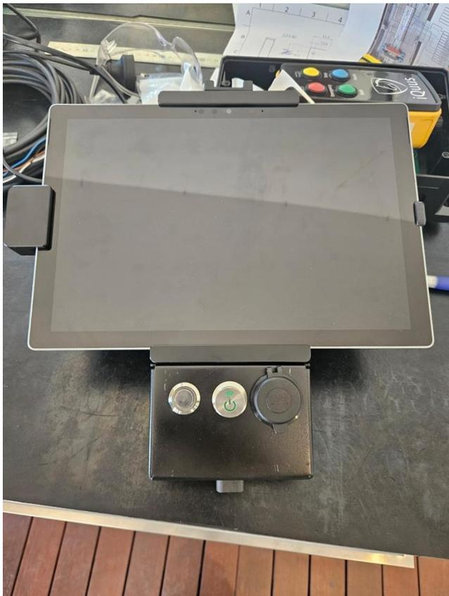
*Picture 6: Iquus tablet with switch bracket installed*
